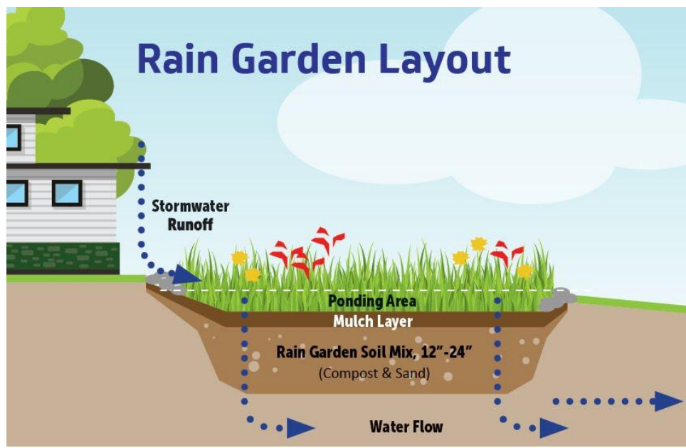
Figure 5: Diagram of a Rain Garden (Courtesy of Hillsborough County Board of Commissioners)
